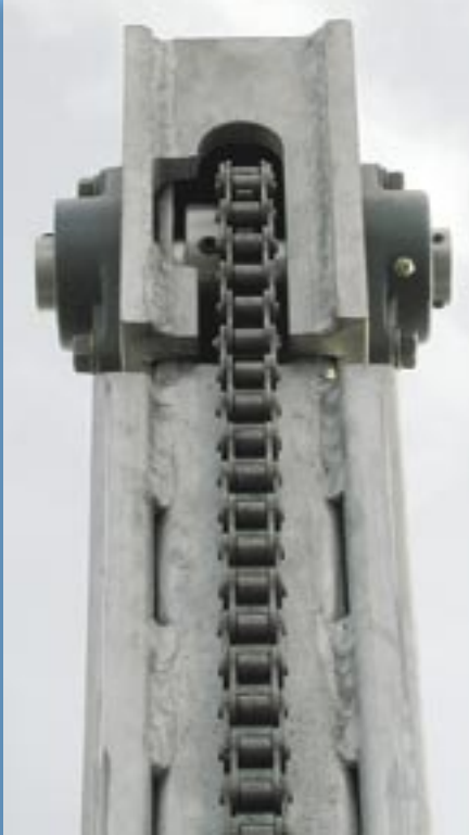
Roller chain over sprocket design feed system includes chain tensioning adjustment.
